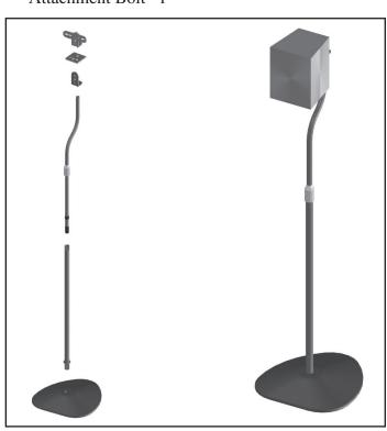
**Step 2:** Thread the end of the Lower Pillar (b) with the Base Nut down into the Base (a). Tighten the Base Nut down onto the Base as necessary, shown in Diagram 2.
